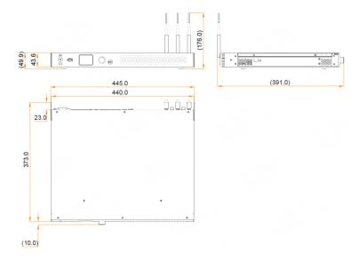
Tolerance: ±0.3 Unit: mm
