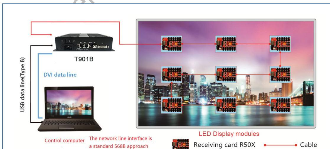
Note: The number of T901 sending card and receiving cards per screen need depends on the screen size.
