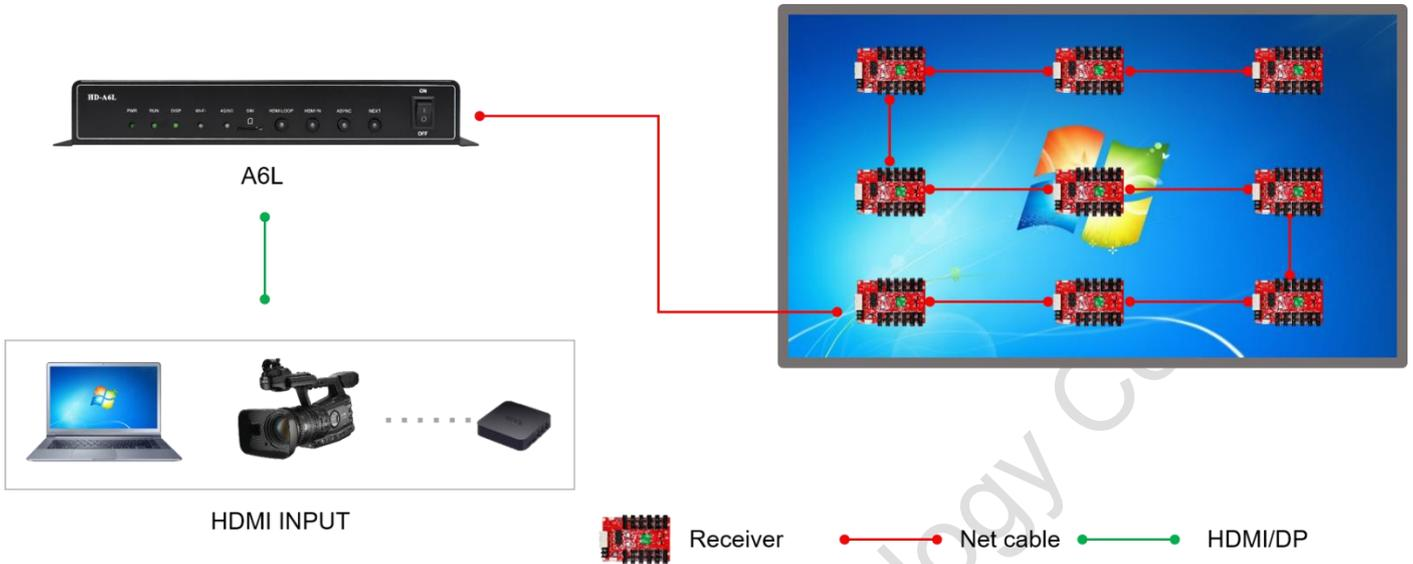
4. Multi-screen splicing application: use HDMI high-definition signal lines to splice in series, and automatically splice the contents of multiple display screens into an overall picture.
