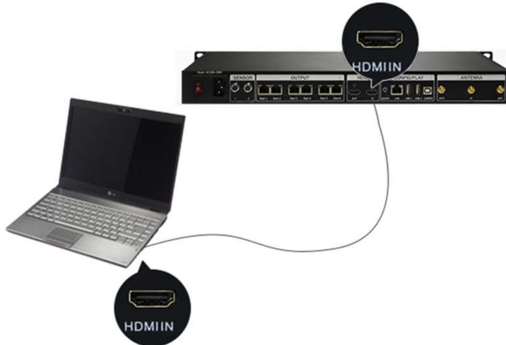
**Note:** C7 will automatically switch to play sync signal program when an external HDMI signal input is detected. You can press [ **Input Switch** ] button to return async signal program playing.
