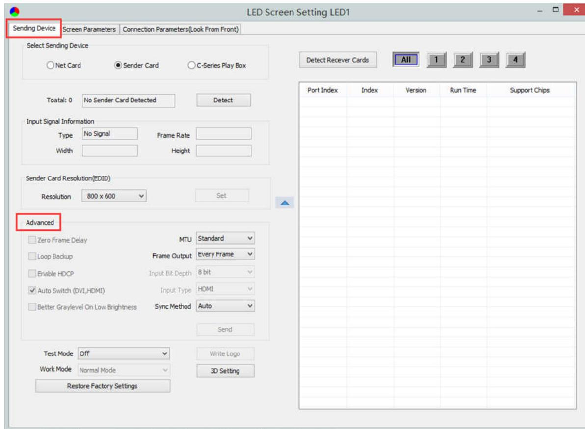
**Sender Card Resolution:** Generally, sender card resolution must be consistent with the graphic card's.
